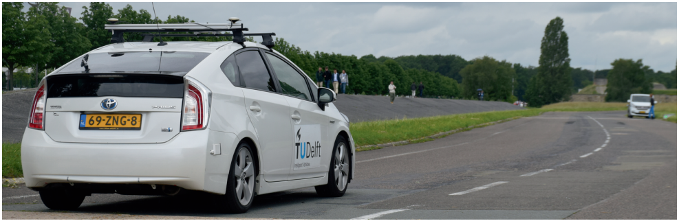
Figure 7.1: The SafeVRU platform for interaction with VRUs on-board the vehicle demonstrator at the start of the pedestrian scenario. The dummy can be seen in the distance on the right.
