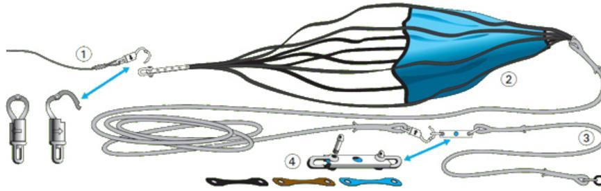
Figure 6.7: The cable parachute of a sailplane cable (Corporaal 2017)
