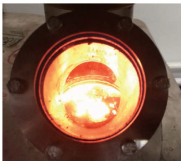
Fig. 3. The event of liquid dripping, viewed from the glass window located at the lower part of the RSM furnace. (Online version in color.)
