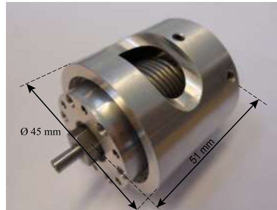
Figure 1. A photograph of the BIC-PEA. It weighs 202 g and fits in a cylinder with a length of 51 mm and a diameter of 45 mm.
