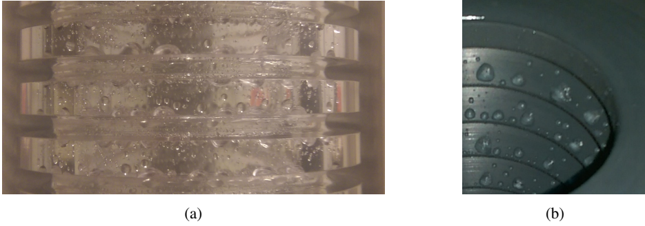
Figure 4.18: Qualitative view of the filling pattern for a corrugated pipe with geometry D after hydrophobic wall treatment (a), and geometry E (b). Liquid addition does not result in an axisymmetric filling in these cases, but rather appears as small patches of liquid inside the cavities.
