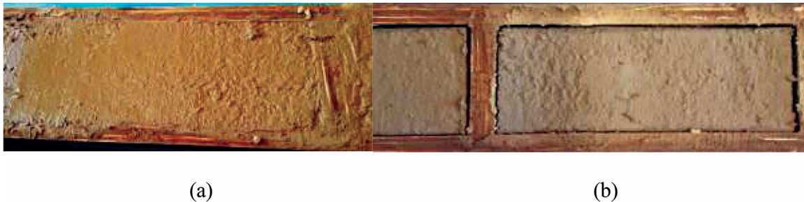
FIGURE 5. Picture of mortar just cast (a) and after five days since pouring (b): volumetric shrinkage of about 18% [26].
