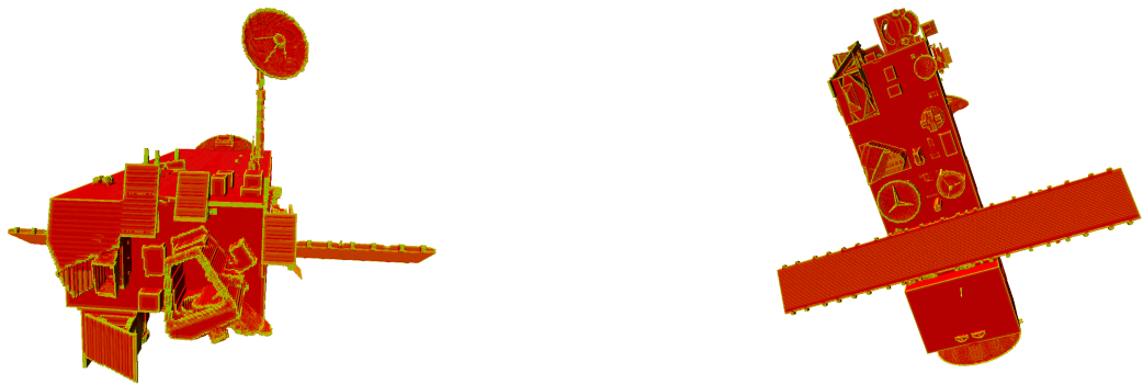
Figure 6.4: Envisat graspability as analysed by voxel superimposition + coplanarity of contact points (#7) with Reward = 1, Penalty = 10, Bin saturation = 50, and Bin steps = 100.
