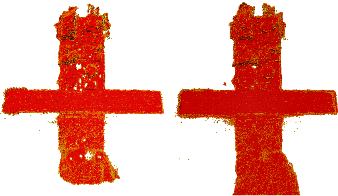
Figure 7.14: Global grasp planning of Envisat (1:10 model) reconstructed from a single point cloud snapshot at a distance of 1.29 m (left) and 10 snapshots at a distance of 1.29–0.82 m (right), voxel leaf size of 0.005 m.
