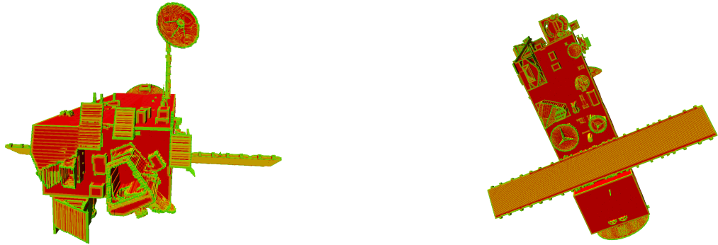
Figure 6.3: Envisat graspability as analysed by coplanarity of contact points method (#5) with Bin saturation = 50 and Bin steps = 100
