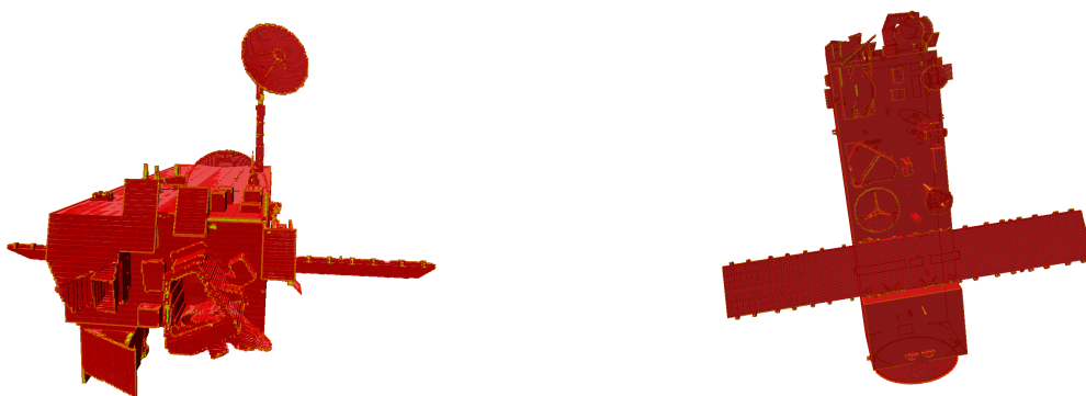
Figure 6.1: Envisat graspability as analysed by voxel superimposition method (#1) with Reward = 1, and Penalty = 50.
