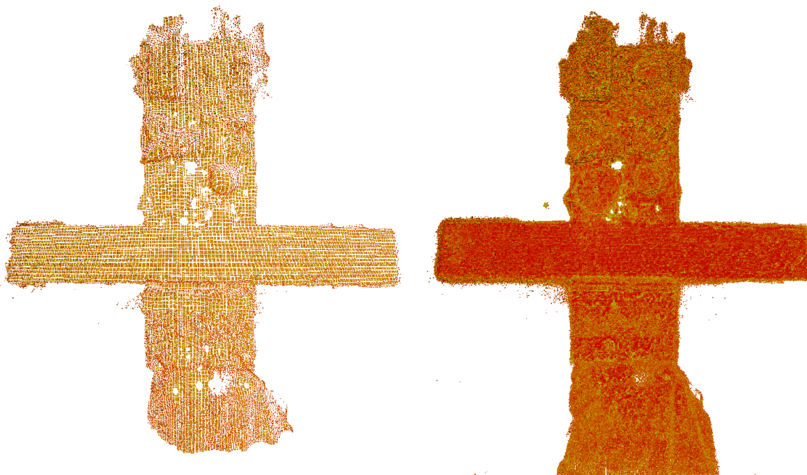
Figure 7.11: Global grasp planning of Envisat (1:10 model) reconstructed from a single point cloud snapshot at a distance of 1.29 m (left) and 10 snapshots at a distance of 1.29–0.82 m (right), voxel leaf size of 0.002 m.
