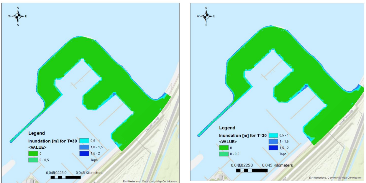
Figure B.2: Inundation maps Parkhaven for T=30 years for a situation excluding (left) and including (right) flexible water level management.
