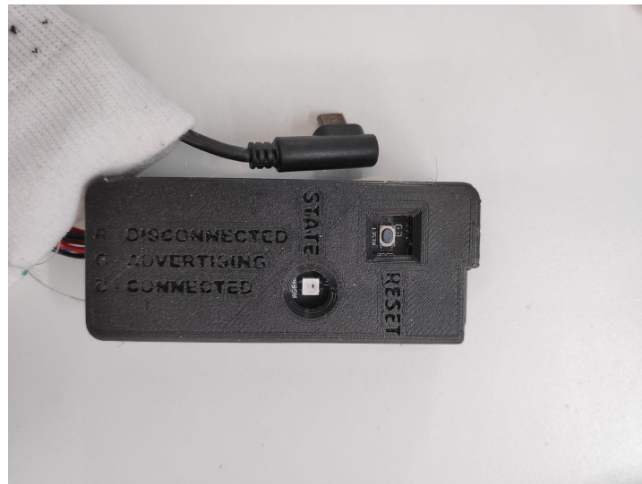
Figure 6.3: The 3D-printed box to house the ESP32, the EDA sensor and the accelerometer
