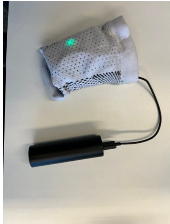
Figure 6.6: The sock attached to the power bank
