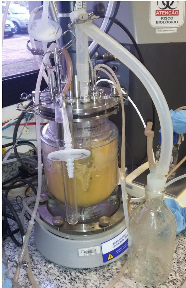
Figure 2.1 – Cellulose feeding method
