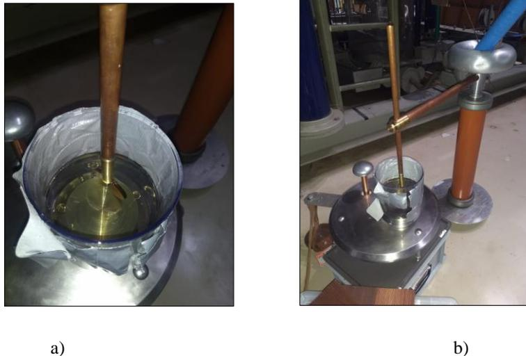
Figure 4. 15 a): Simulating surface discharges in oil under impulse voltage b): test sample under impulse voltage
