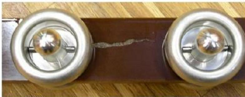
Figure 1. 4: Creepage discharge in mineral oil [5]
