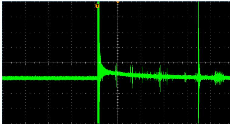
Figure 4. 27: Current noise signal without winding installed at 200 kV(current- 2V/div; time-40 $\mu$ s/div)
