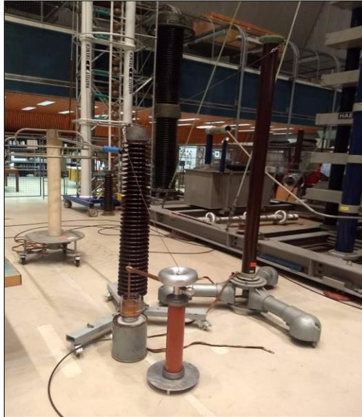
Figure 4. 1: Initial test set up for electrical streamer detection in ester under LI voltage
