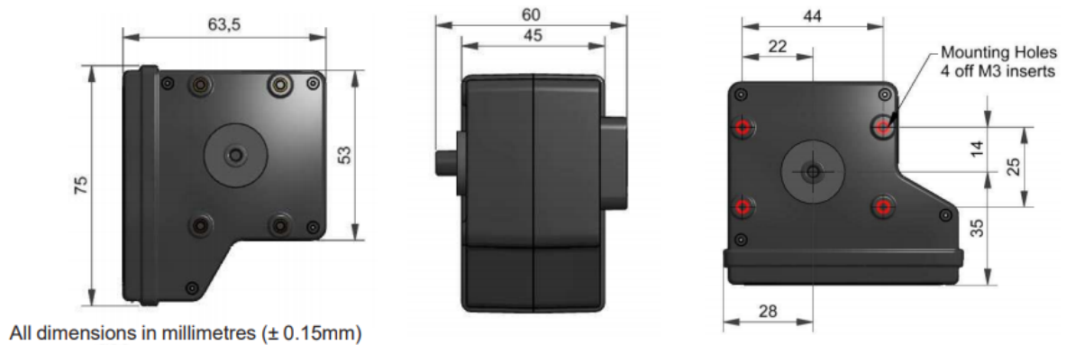
Figure 6.21: Dimensions of a PM sensor (Alphasense, 2018)
