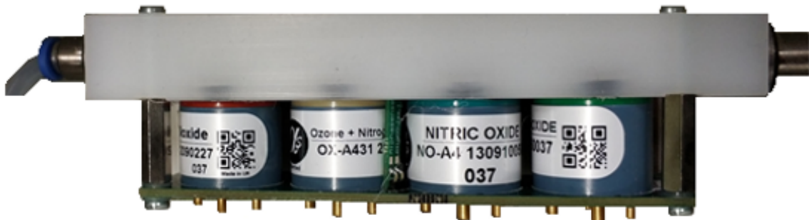
Figure 6.19: Sensors of the SensaBox (own composition, 2018)
