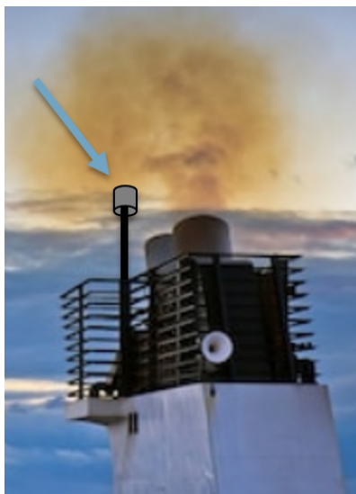
Figure 5.3: Example of location in the exhaust plume (own composition, 2018)
