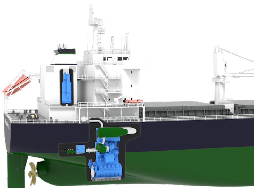
Figure 4.1: Ship including SCR, EGR and scrubber installation (DNV-GL, 2018a)
