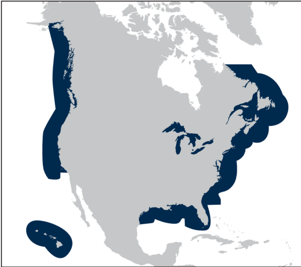
Figure A.2: The North American ECA 200 nautical miles offshore US and Canada, including Hawaii, St. Lawrence Waterway and the Great Lakes (American Bureau of Shipping, 2018)
