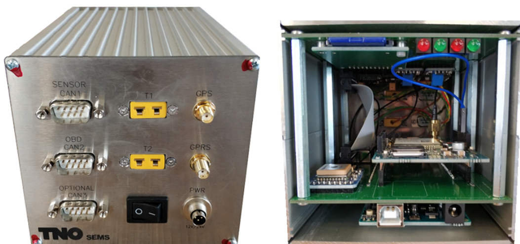
Figure 6.15: Smart emission measurement system (own composition, 2018)
