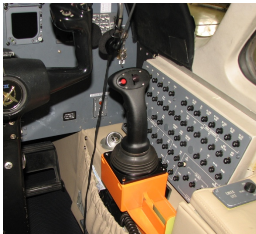
Figure 6. Experimental fixed force side stick.
