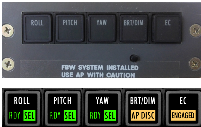
Figure 5. FBW Control Panel
