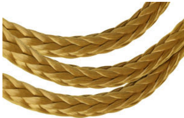
Figure 4.26: Flat Zylon ® braids used for sailboats
