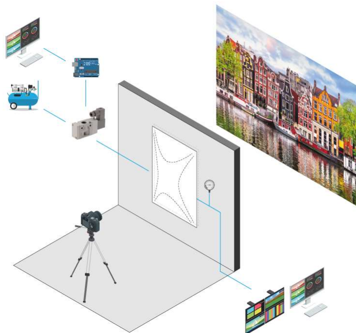
Figure 68: Optical test setup for analysis of distortion of exterior view with camera to capture HDR images for objective comparisons.
