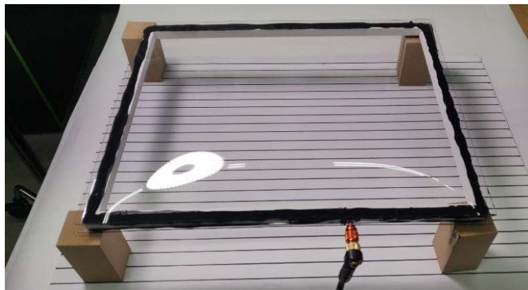
Figure 27: PMMA prototype with added air pressure in the cavity.
