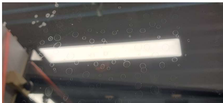
Figure 42: Safety films applied on the full size panels showed bubbles and marks even after 2 attempts.
