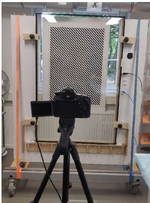
Figure 55: DSLR camera setup in front of the glass panel, and zebra board behind.
