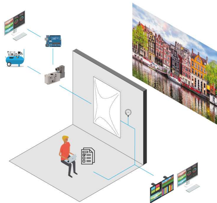
Figure 69: Subjective test setup for analysis of effect of distortions on occupant satisfaction with a single volunteers or groups of volunteers recording their perception towards deforming glass.
