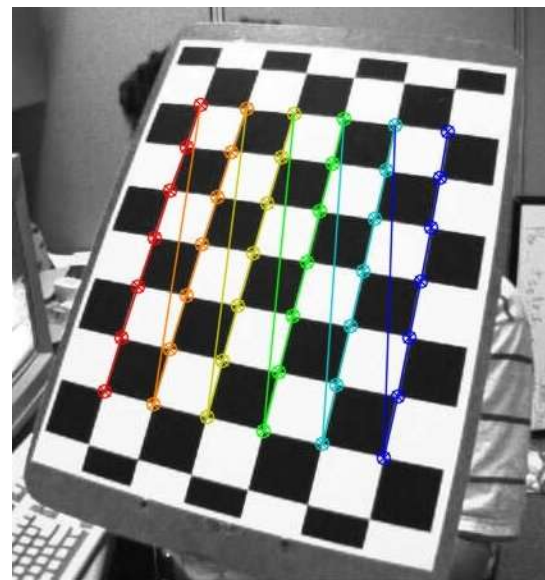
Figure 54: Use of checkerboard for detecting points for calibration of image using OpenCV library in Python. Source : https://docs.opencv.org/4.x/dc/dbb/tutorial_py_calibration.html
