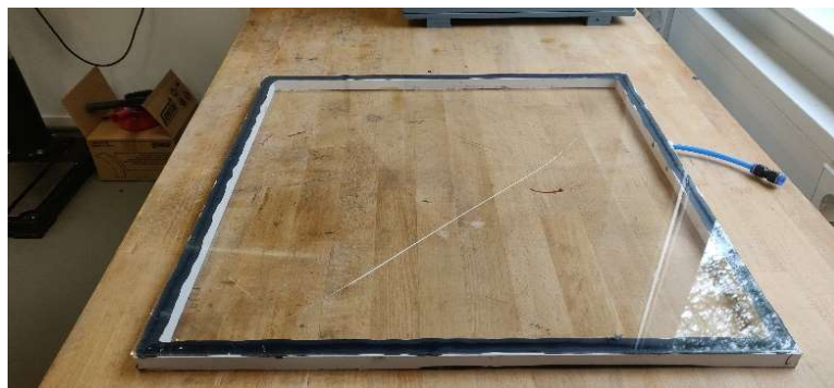
Figure 29: Prototype in aluminosilicate thin glass (AGC Falcon, 1.1mm thick) showing a linear crack after undergoing a breaking test with safety film.
