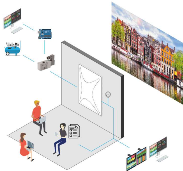
Figure 70: Subjective test setup for analysis of effect of distortions on occupant satisfaction with a single volunteers or groups of volunteers recording their perception towards deforming glass.
