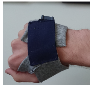
Figure F.4: Second prototype of the interface, the elastic band in combination with the Velcro® strap allow for easy donning and doffing of the interface. The transmission can be attached through a hole at the side of the interface
