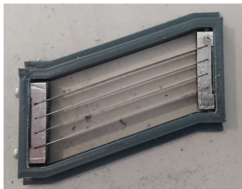
Figure J.1: Flexures and the reinforced mounting block attached to the frame used for keep the position of the mounting block fixed during insertion of the flexures.
