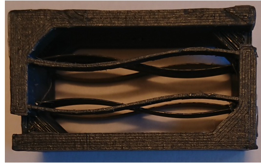
Figure J.3: Prototype of the monolithic negative stiffness mechanism using inclined flexures in its deformed state
