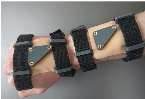
Figure F.3: First prototype of the interface, the mounting holes can be used for the attachment of a transmission
