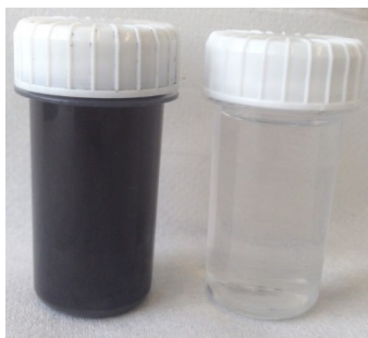
Figure 1. Color of the liquids obtained after milling with and without a surfactant.
