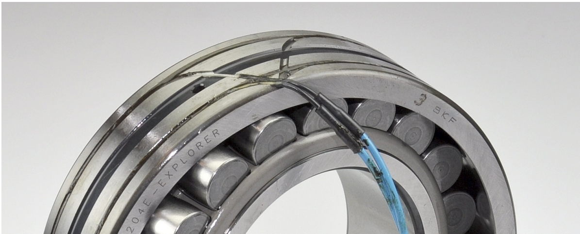
Figure 3.6: Illustration of the outer ring groove including fibers
