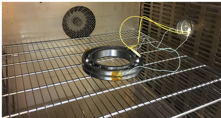
Figure 5.9: Gusto bearing placed in the middle of the Heraeus 0914 oven
