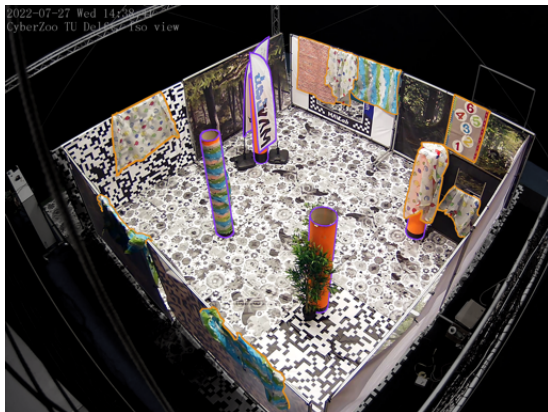
Fig. 9: Overview of the cluttered, obstacle avoidance environment. Obstacles are outlined in purple, while texture-enhancing mats and curtains in orange.
