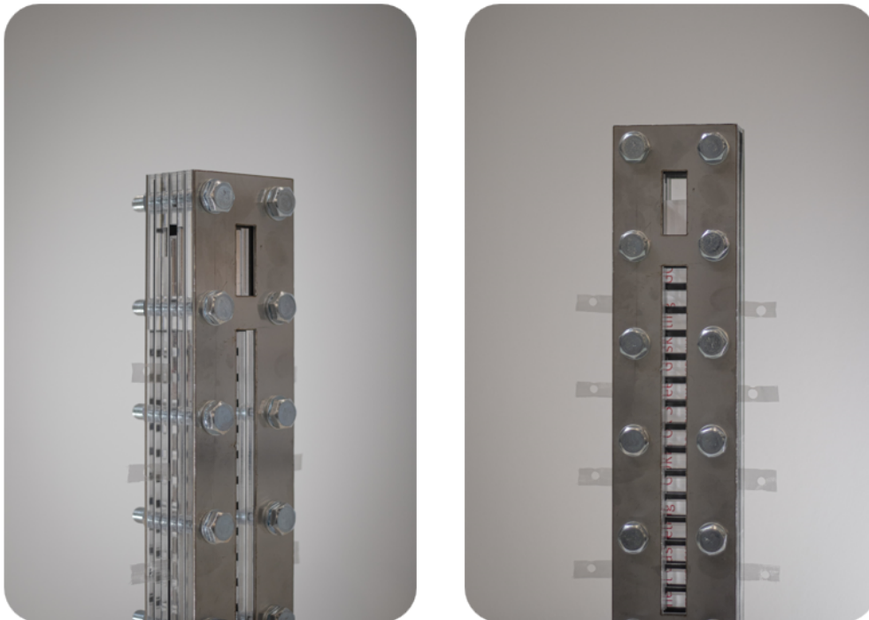
Figure 3.10: Design of the segmented capillary-fed electrolyzer. Left: Isometric side view, showing the inlets to the reservoirs. Right: Front view.
