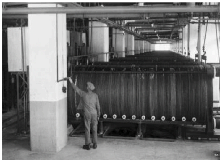
Figure 2.2: Hydropowered water electrolysis plant for production of hydrogen for ammonia synthesis. [17]
