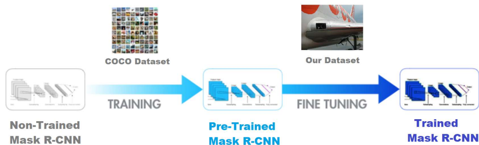
Figure 5: The concept of transfer learning with a warm restart
