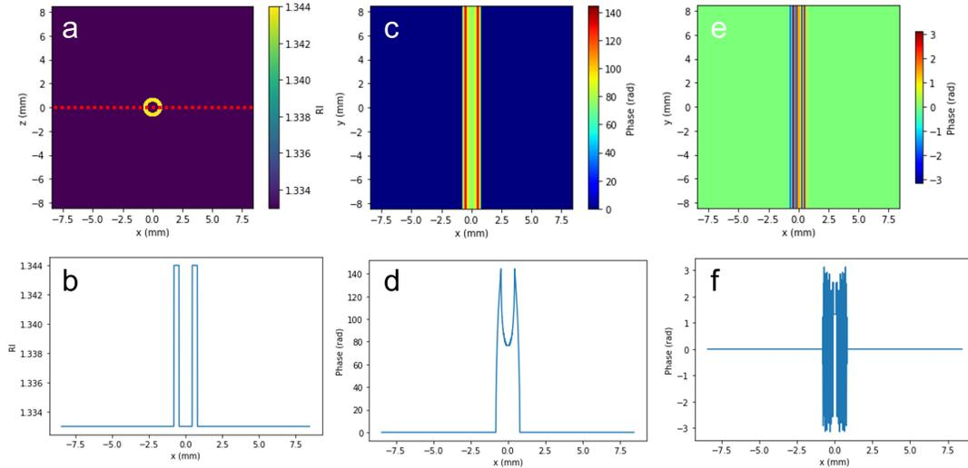
Figure 1. (a) RI distribution of a capillary tube, (b) RI variation along the red line in (a), (c) Ground-truth phase distribution of the capillary tube, (d) Phase distribution of the capillary tube along  $y = 0$  in (c), (e) Principal phase distribution of the capillary tube in (c), (f) Cross-sectional phase variation along  $y = 0$  in (e).
