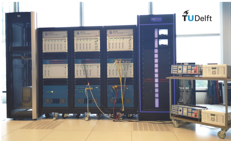
Figure 2.10: Digital power system simulator interfaced with PMUs as HIL via digital to analogue converter outputs and current and voltage amplifiers.
