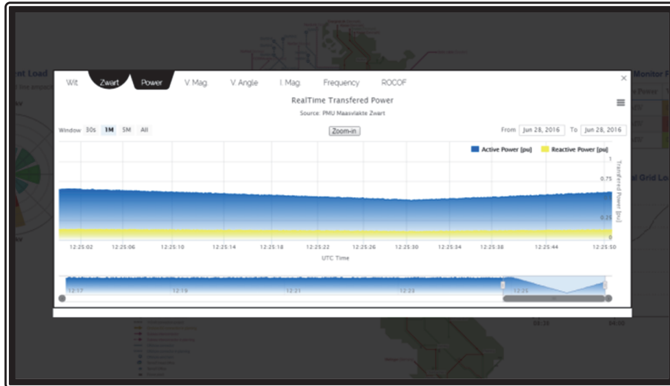
Figure 2.12: Real-time monitoring of active and reactive power.
