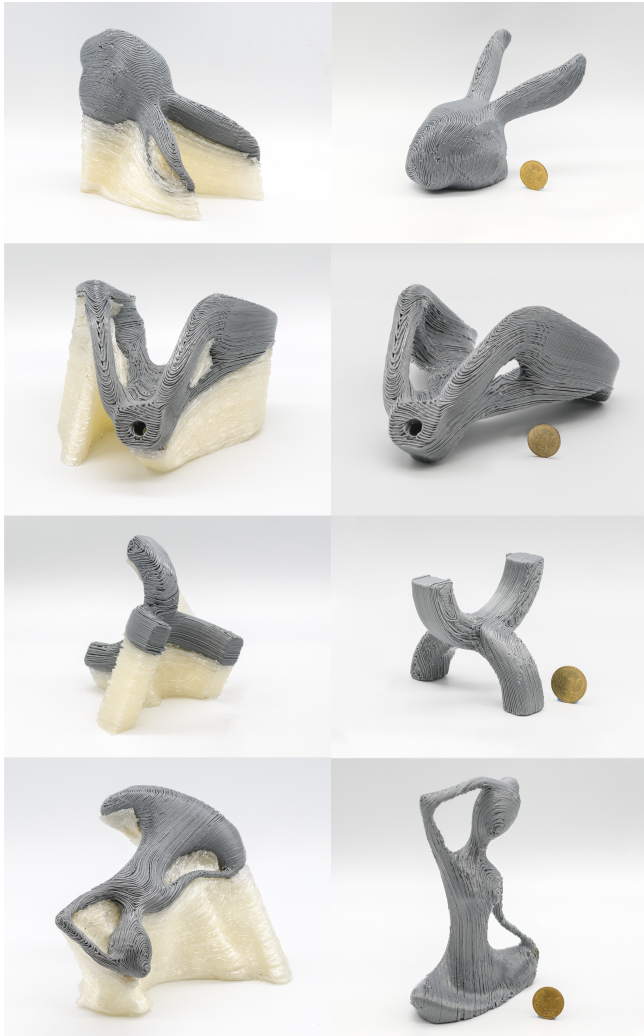
Fig. 14. Physical fabrication results (before and after removing the supporting structures) for Bunny head, Topo-opt, C 2 -model and Yoga.
