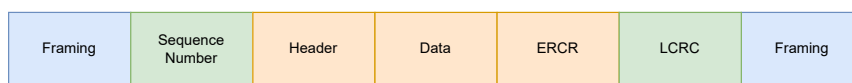
Figure 2.6: Data encapsulation in PCIe: Blue is Physical Layer, Green is Data Link Layer and Orange is Transaction Layer
