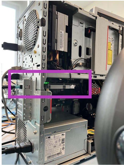
Figure 5.3: Host PC used for the experiments, with the PCOA card by Samtec into a PCIe slot.
