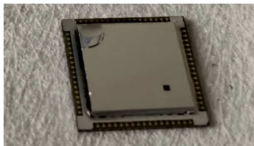
Figure 1: Single 10x10 mm quadrant sensor chip before packaging with cyanoacrylate glue on the top left. Note that this is a multi-project chip and the actual sensor is located at the bottom right under the opening in the metal mask.
