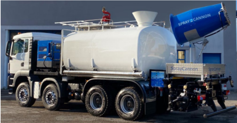
Figure 25: SprayCannon mounted onto truck (MB Dustcontrol, 2022f)
