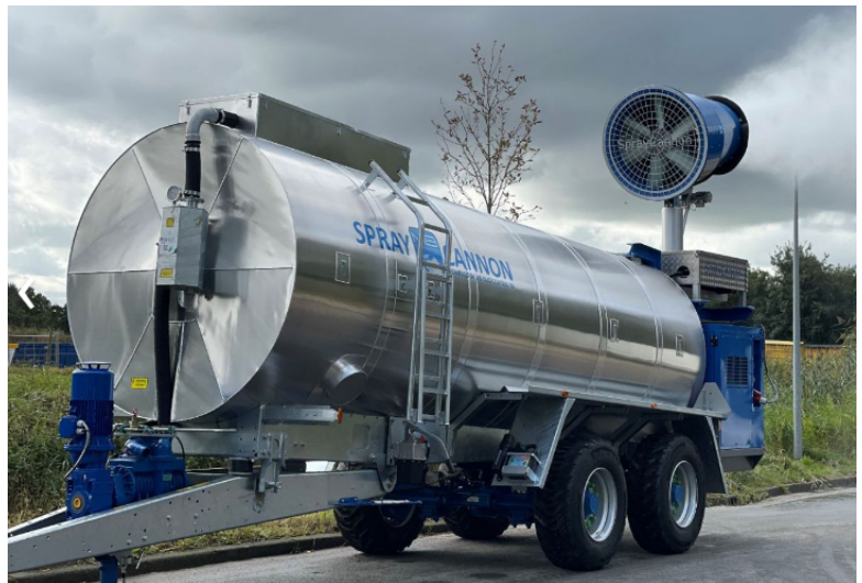
Figure 24: SprayCannon mounted onto tank trailer (MB Dustcontrol, 2022c)
