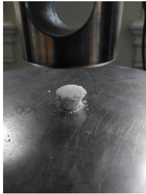
Figure 32: The bone sample before (left) and after (right) the compression test. The samples are compressed by a rate of 1mm/minute in axial loading.
