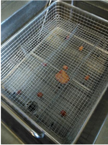
Figure 29: The ultrasonic tank with basket and bone samples prior to cleaning.
