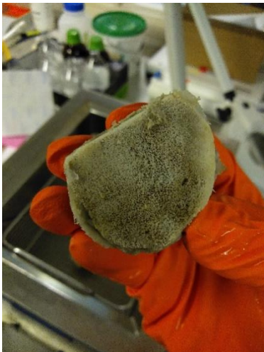
Figure 33: A porcine femoral head after treatment with acetone and isopropanol according to the processing protocol in chapter five. Only the surface of the bone is partly cleaned by these chemicals.
