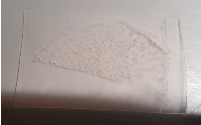
Figure 30: Cutting plate of bone sample 56575 clean at 130 kHz.
