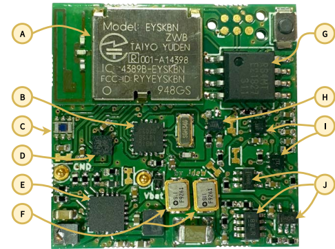
Figure 7: FreeBie mote (front side). A total size is 1”×1”. Components marked as (A)–(J) are explained in Section 4.
