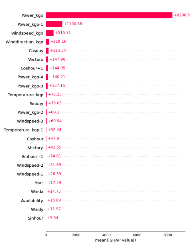
FIGURE 4.2: Mean SHAP values of the wind input variables calculated using the tree regressor XGBoost.
