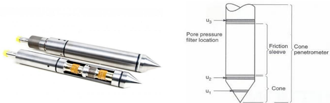
Figure 2-18: Cone penetrometer with resistance parameters from (Lunne, et al., 1997)
