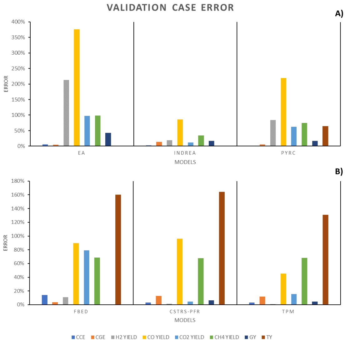
Figure 35. Summary of the relative error of the equilibrium models (A) and the kinetic models (B) at ER=0.25 and T=877°C.
