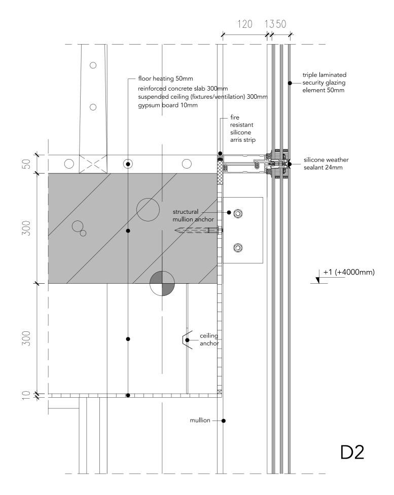
suspended ceiling (fixtures/ventilation 300mm)
