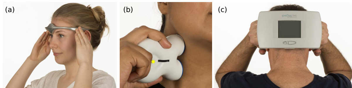
Figure 2.2: Different non-invasive stimulation devices. a) Cefaly device for supraorbital stimulation to suppress episodic migraines. b) gammaCore device for vagus nerve stimulation, used to prevent cluster headache attacks. c) SpringTMS device for transcranial magnetic stimulation of the occipital region for the prevention of migraine attacks. Modified images taken from [6]
