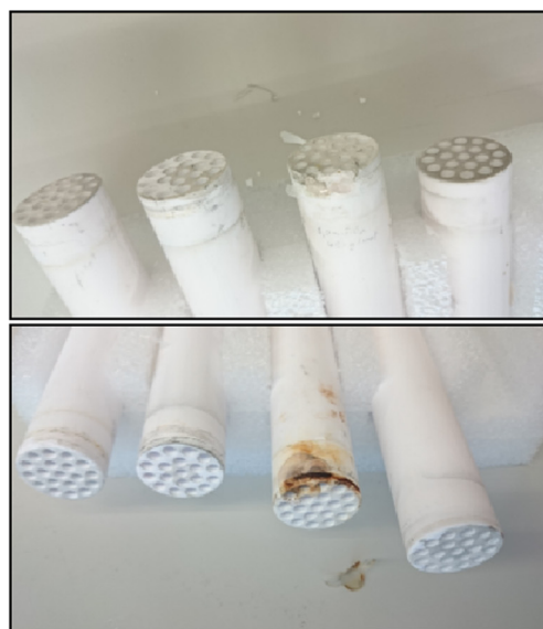
Fig. 4. (a) Permeability in time during ceramic NF using model sewage with and without interval hydraulic backwash performed with the configuration with large membranes. Hydraulic backwash was applied at 6 bar pressure for 5 min when the permeability had reached 10 \text{ L} \cdot (\text{m}^2 \cdot \text{h} \cdot \text{bar})^{-1} . (b) Pictures of damage of the ceramic NF membranes after hydraulic backwash was applied. The layer on the edges of the membrane were damaged. Therefore, the feed water can flow directly to the permeate via the support layer of the membrane.
