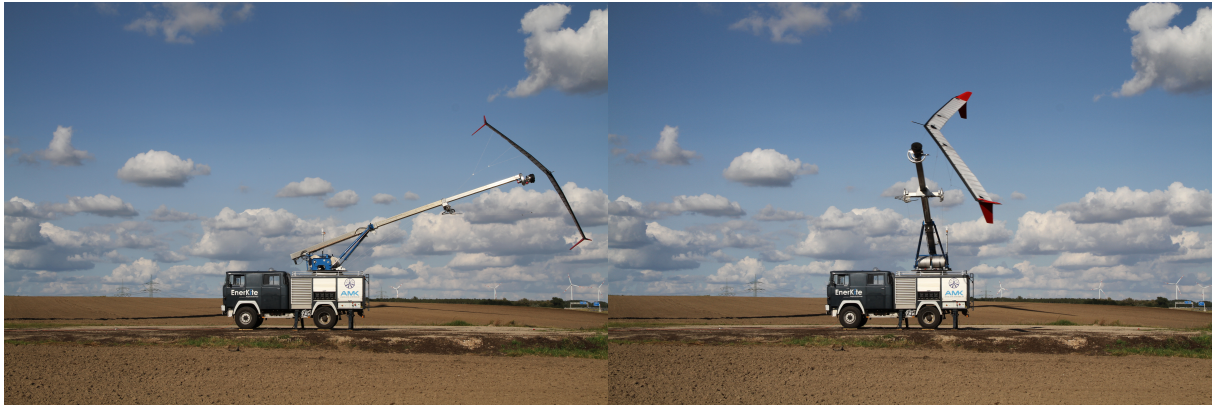
Figure 1: EnerKite technical demonstrator system comprising a mobile base station with a rotational landing and launching mast, pictured during a launching operation with a prototype wing.
