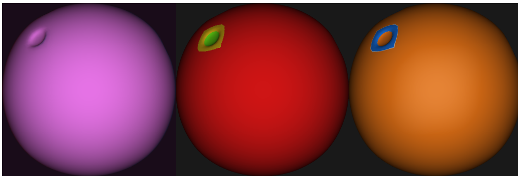
Fig. 5.6.: Model 'dented sphere'. Left: rendered with phong shading, for reference. Middle: segmentation, 3 segments. Right: Gaussian curvature, orange is positive, blue is negative.
