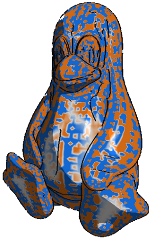
Fig. 4.18.: On certain meshes, the computed discrete Gaussian curvature has a lot of noise
