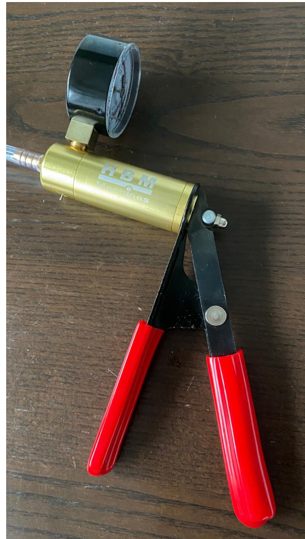
Figure 5.2: The vacuum pump that is used in this study
