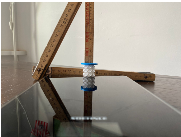
Figure A.14: Measuring the lattice force and deformation (Extended)
