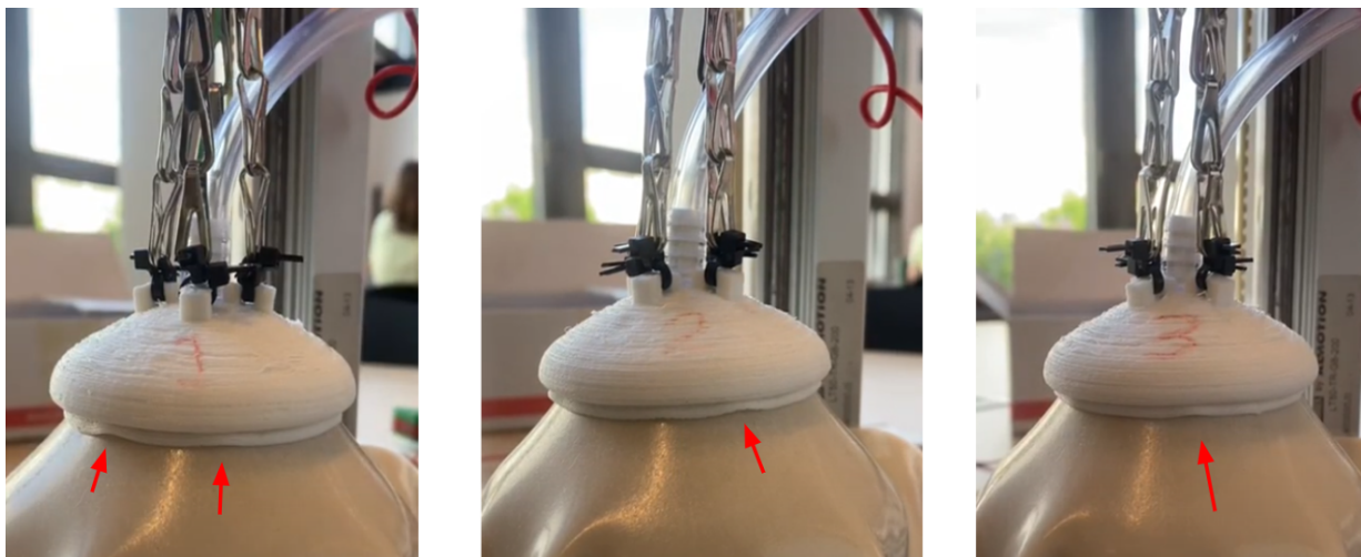
Figure 5.16: Observation of a curling lip immediately prior to detachment. The images from left to right correspond to Model 1, Model 2, and Model 3. The red arrows indicate the location of the sealing lip that curls which result in leakage of negative pressure
