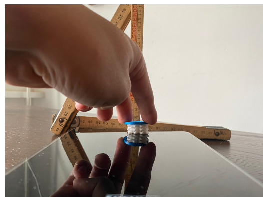
Figure A.15: Measuring the lattice force and deformation until no light can be visually be seen (Compressed)
