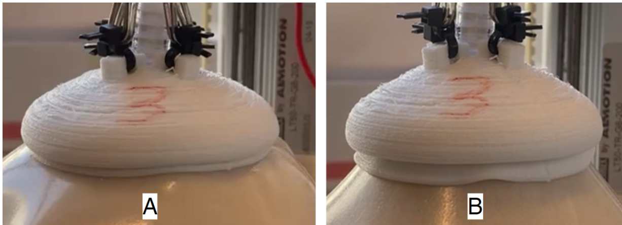
Figure 5.15: Deformation of the suction cup. (A) The suction cup before the application of traction force, and (B) the suction cup prior detachment. The images illustrate the deformation of the entire cup during experiment 1.
