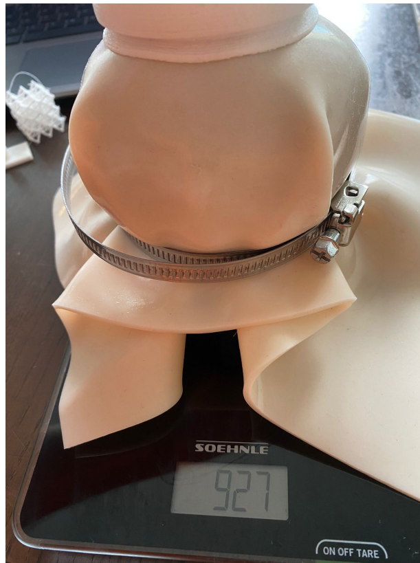
Figure A.13: Measuring the force that is needed to form a seal with the infant surrogate surface.
