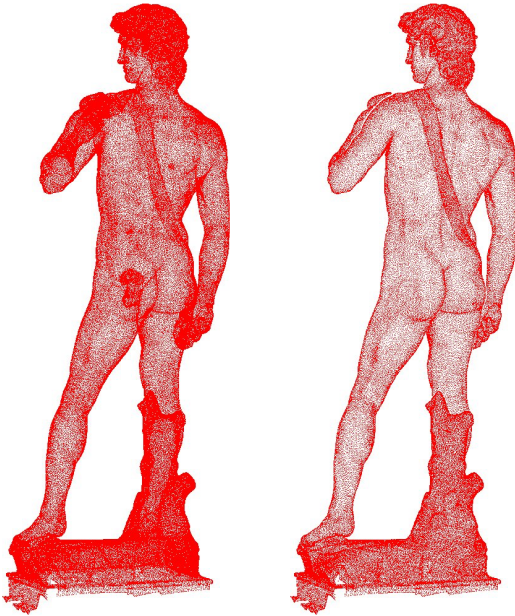
Figure 2.3: Images taken from Katz, Tal, and Basri (2007). A point cloud of Michelangelo’s David ; on the left the input to the Hidden Point Removal operator, on the right the output
