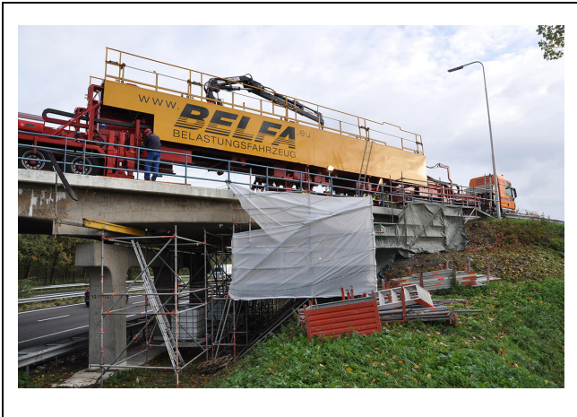
Figure 1. The German BELFA load testing vehicle on the Vlijmen-Oost viaduct in the Netherlands. Reprinted with permission from (1).
