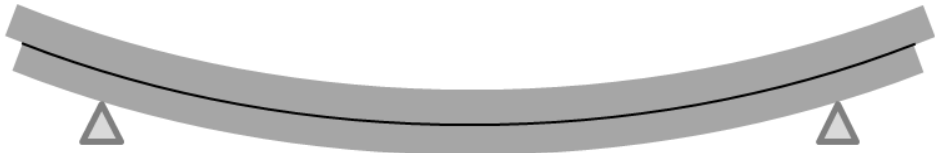
Figure 3.12 Slip between two beam sections without shear transfer in the longitudinal joint
