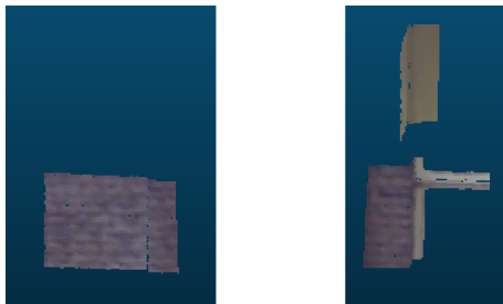
Figure 4.2: On the left, the result of a line of sight can be seen from the reference position, which is the position of the scanner in this case, towards a facade, which has only a single group of points. On the right, the result of a line of sight can be seen of the edge of a hole in the facade and as can be seen here, there are multiple groups of points indicating a higher variance in the distances of points towards the reference position for this line of sight.
