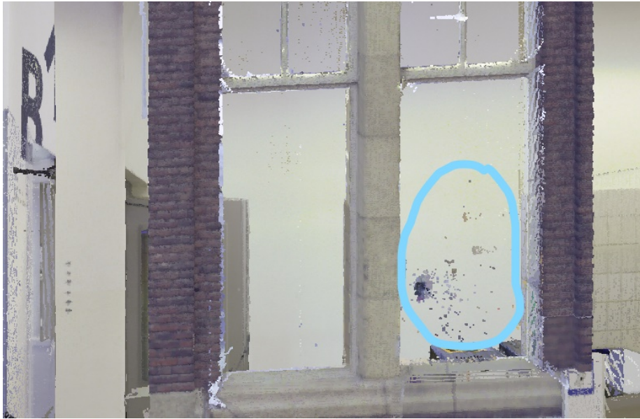
Figure 3.5: Example from the test scene used in Chapter 5 where points are captured directly on glass, here being the blue and grey points in the right window.
