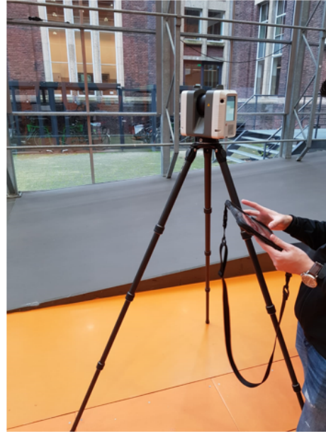
Figure 5.1: The Leica RTC360 3D laser scanner is used for Terrestrial Laser Scanning during this thesis 10 .
