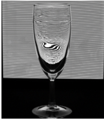
Figure 2.2: Example of Active Illumination. Structured light with a striped pattern is projected onto the glass. By registering the distortions of the pattern the location of the distortion source, in this case the drinking glass, can be deduced. 2
