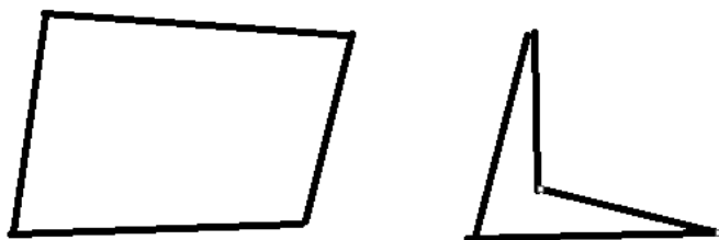
Figure 4.9: The shape on the left shows a close to perfect rectangle which will be detected by the algorithm as its errors in the corners stay within the error margin for each corner. The shape on the right fulfils the 4 points requirement but does not stay within the error margin for its corners and is therefore not labelled as a window candidate
