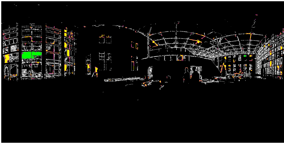
Figure 5.16: Rectangle validation with an error margin of 15 degrees. Only 3 contours are labeled as candidate windows here which is too narrow.
