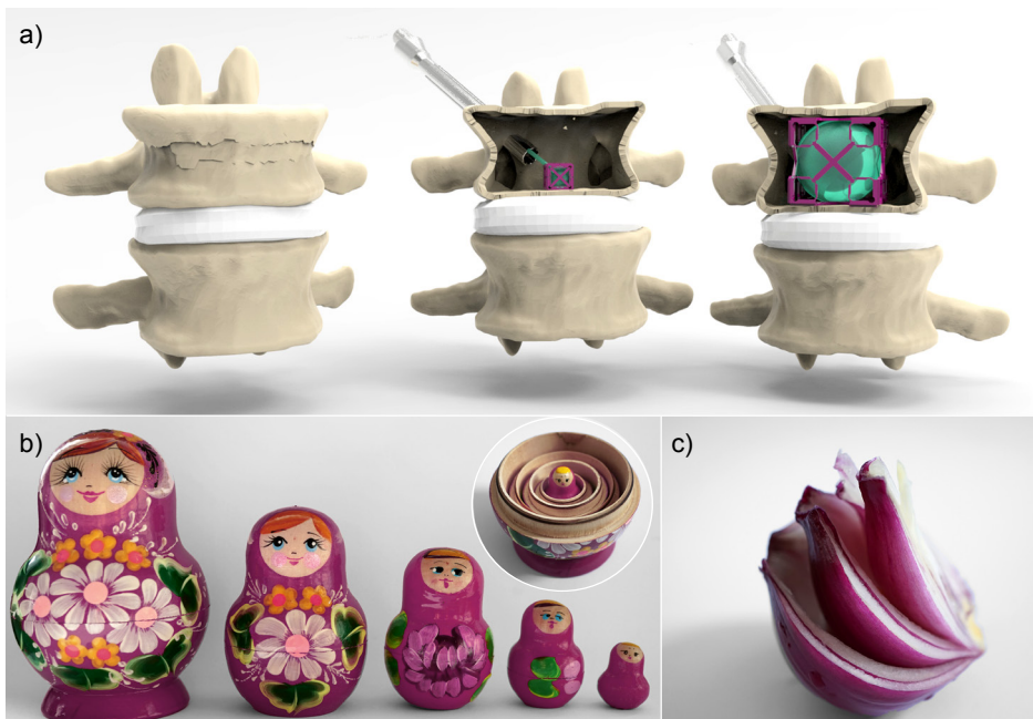
Figure 1. a) The novel concept of deployable implants as applied to the treatment of a fractured vertebra. With minimally invasive surgery, a deployable structure including a balloon is placed inside the fractured vertebra. Upon the inflation of the balloon, the deployable structure expands and restores the height of the vertebra. The balloon is then removed. b) Russian dolls shown from the front and top views. c) Red onion also consists of different layers.
