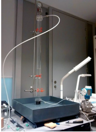
Figure 2: Permeability experiment set-up: Left: picture of the set-up. Center: Schematic overview 1. vacuum pump, 2. air valve, 3. water column, 4. water, 5. pressure gauge, 6. sample holder, 7. water container, 8. sample. Right: pressure difference over the sample [Pa], with h - water level within the column [m], L - Length of the sample [m], \rho - density of the water [kg/m 3 ], g - gravitational acceleration [m/s 2 ], P_{atm} - atmospheric pressure [Pa], v - fluid velocity within the column [m/s]. The kinetic terms ( \frac{1}{2} \cdot \rho \cdot v^2 ) is negligible because this term is relatively small compared to the pressure applied by the water ( \rho \cdot g \cdot h ).
