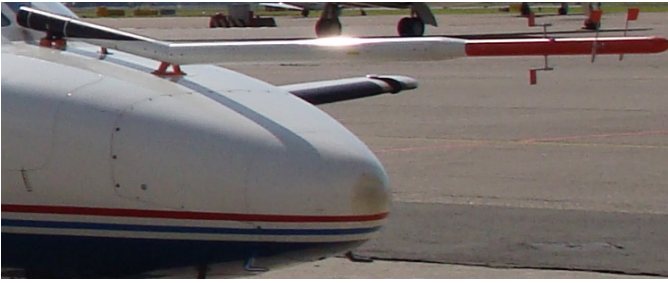
Figure 2.6: The vanes on the boom for measuring the angle of attack and angle of sideslip. Photo credits by Daan Pool.
