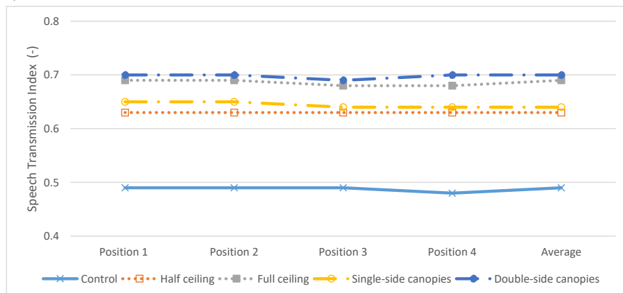
FIG. 6.7 Acoustic simulation results in different positions in the instruction situation.
