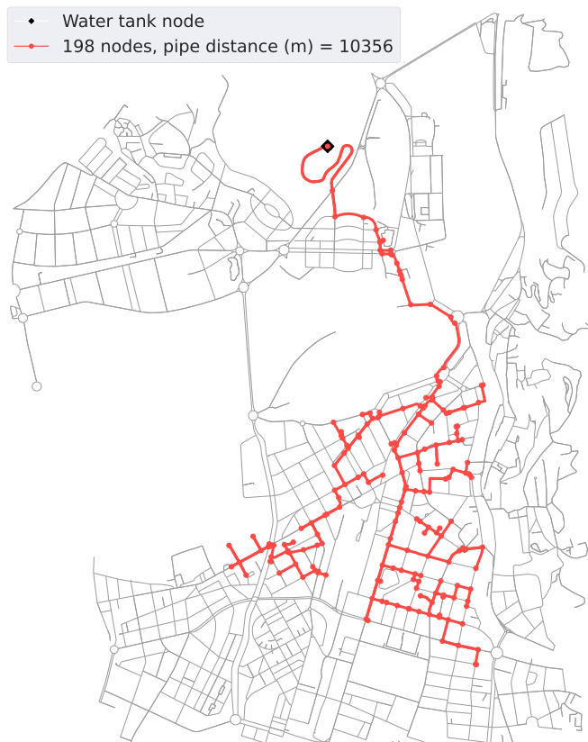
Fig. 3. Visualization of the ‘non-resilient’ current reclaimed water network in Girona (highlighted in red) overlaying the Girona street graph (in grey).
