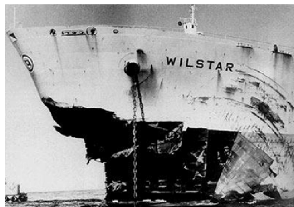
Figure 1.4: Damaged bow of the Norwegian tanker Wilstar (Kharif et al., 2009)
