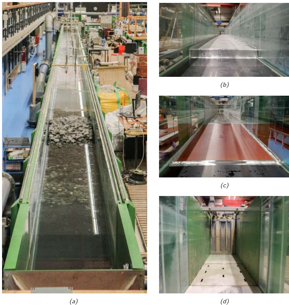
Figure 3.3: Impression of the flume set-up at the Delft University of Technology Hydraulic Engineering laboratory. (a) Is an overview of the flume. The picture is taken at the end of the flume. (b) Shows the step. (c) Shows the slope. (d) Is a front view of the paddle board.
