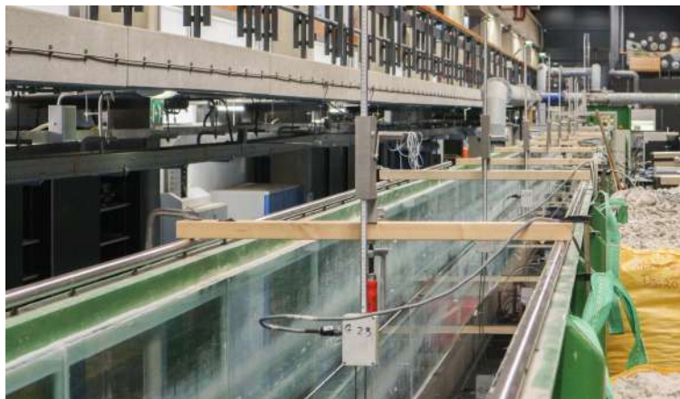
Figure 4.1: Impression of the set-up for the assessment of the second-order generation at TU Delft
