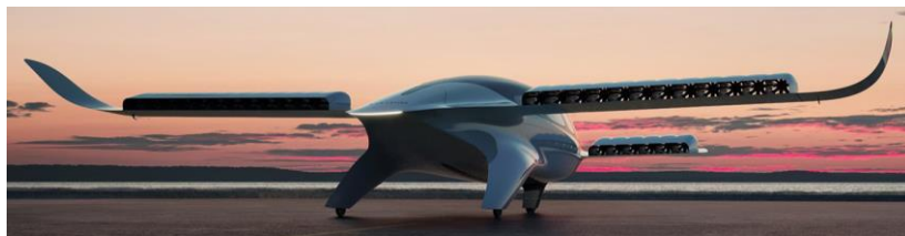
Lilium Jet, vectored thrust with fixed wings configuration, by (Lilium, 2021)
