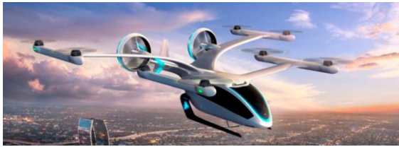
Embraer's EVE, lift + cruise configuration, by (EmbraerX, 2021)
