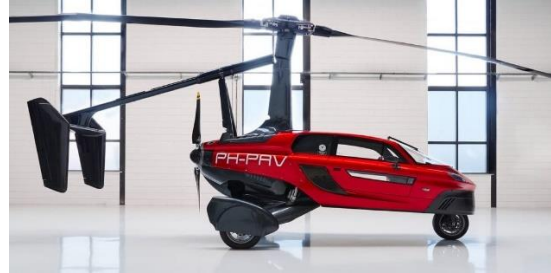
PAL-V International Liberty, gyrocopter configuration, by (PAL-V, 2021)
