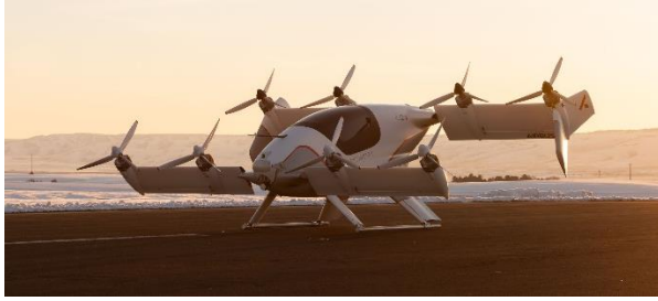
Airbus Vahana, tilt wing configuration, by (Rodriguez, 2019)
