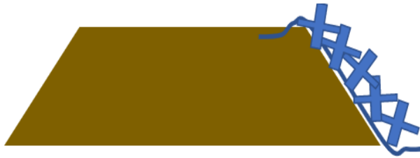
Figure 45 Concept sketch geotextile with armour layer
