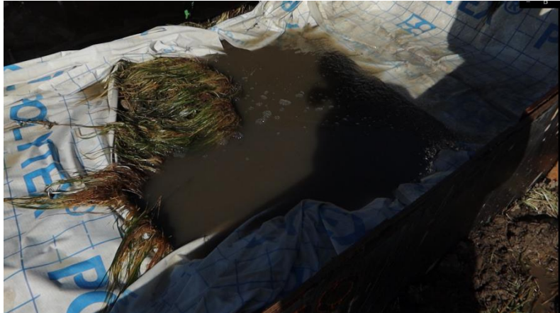
Figure 25 Torn off sheet at lower damage after overflow tests with 1m tear through both sheet layers
