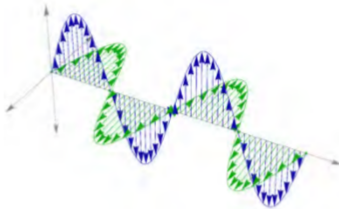
Figure 2.2: Generic orthogonally polarized waves.
